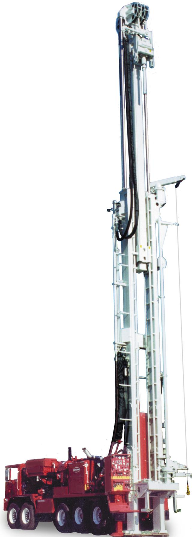
**CARRIER MOUNTED RIG EQUIPPED WITH TELEMAST**
