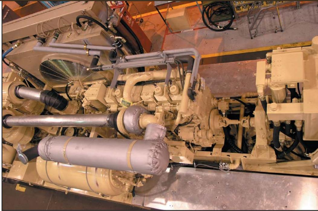
The engine, compressor, and hydraulic pumps are mounted on a floating power pack base rather than directly onto the chassis mainframe. This arrangement assures proper alignment of power components and decreases wear.
